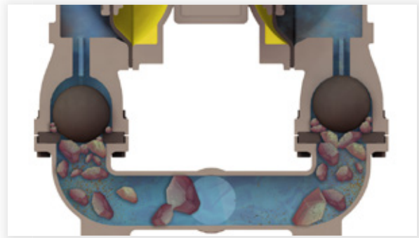
Large solids cannot pass through pump, affecting operation
